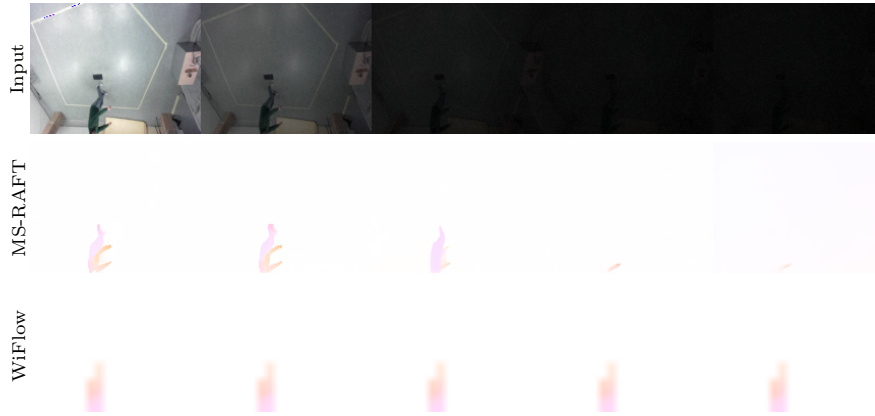
Fig. A.2. Brightness dependency of MS-RAFT and our \text{WiFlow}_{\text{Combo}} . We gradually decrease the brightness and add additive noise to the original frame. Accuracy of MS-RAFT decreases while \text{WiFlow}_{\text{Combo}} is not affected, as it is independent of the input images.
